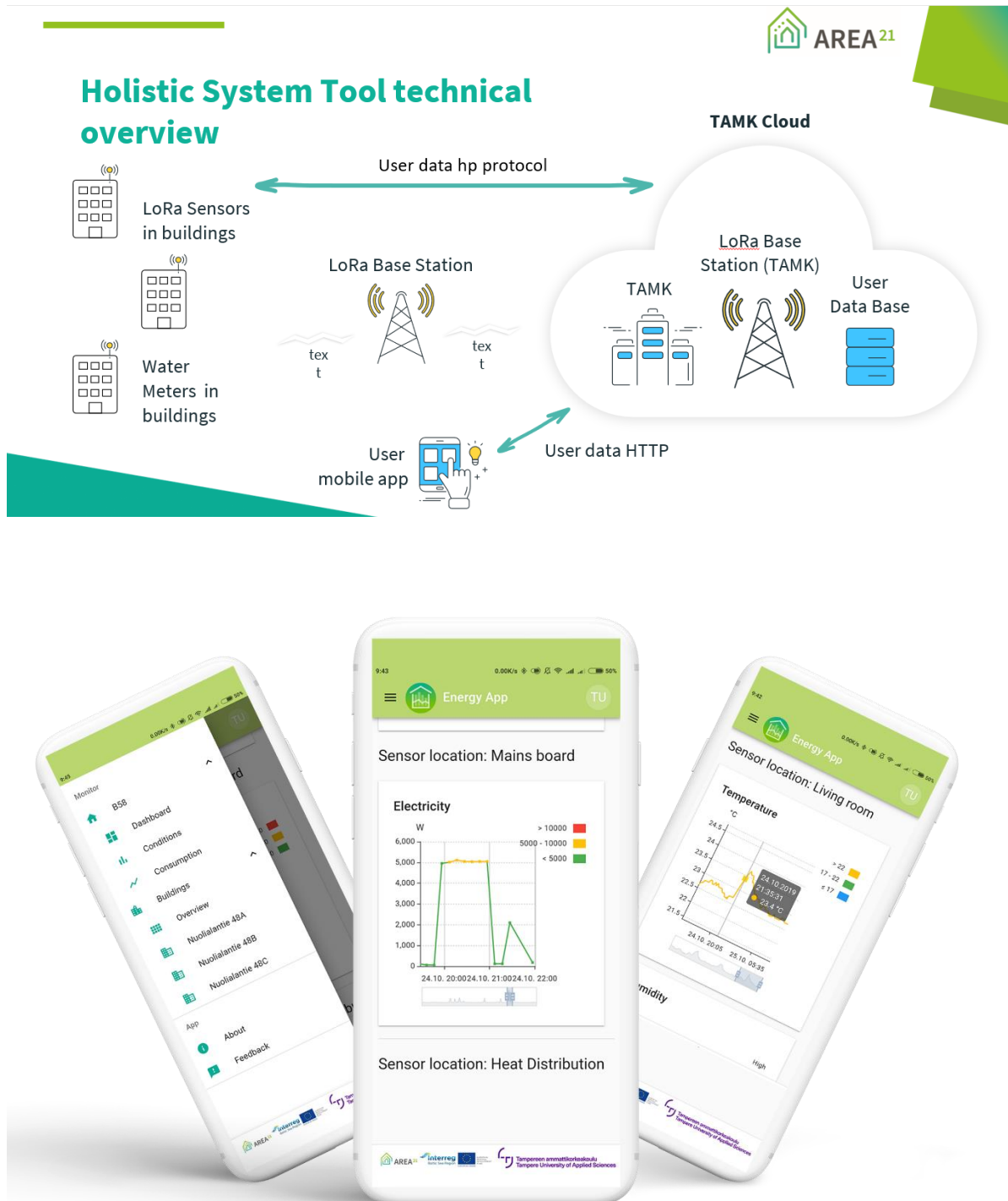
Figure 2. The system overview and mobile application interfaces of the real-time energy monitoring tool (Source: AREA 21 project)
